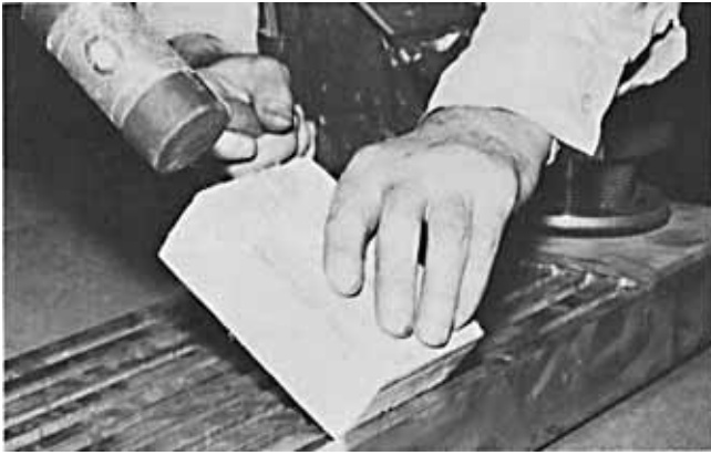
FIG. 27 Straightening tubes with a wooden block & mallet
