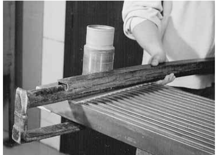
FIG. 25 Locate twisting hook as close as possible to the nipple or stud
