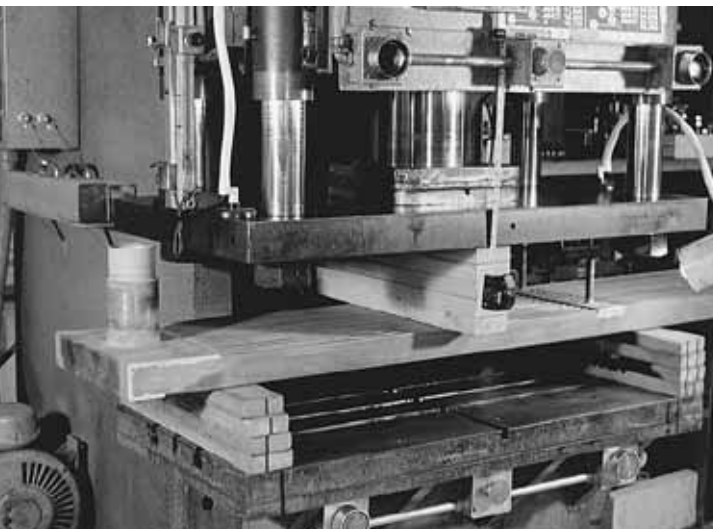
FIG. 24 Creating a bend in a cooler using a hydraulic press
