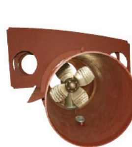
Customised tunnel with ready-made frame sections.
